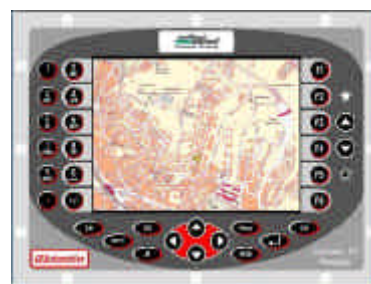
Fig. 5.14: The In Vehicle Terminal of DRT service
